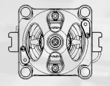
Application specific mounting plate with rubber grommets for vibration damping
